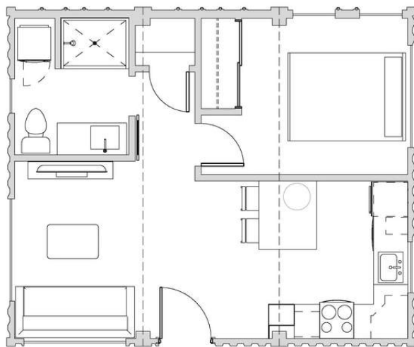
Three containers (no storage loft)
